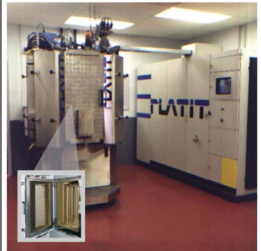
Our new advanced coating system represents the highest standard of modern hard coating technology for tools and wear parts. It is unequalled in both coating quality and long term coating process reproducibility. The revolutionary Platit Linear-Arc-Concept, with a new type of arc control (MAC), magnetic arc confinement allows maximum coating flexibility, efficiency and guarantees incomparable production consistency and coating performance.
